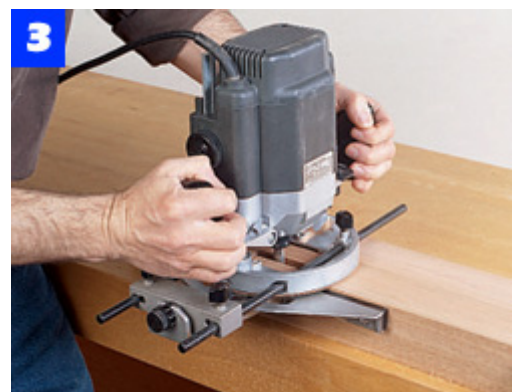
Route the mortises in the legs. Clamp a second leg to the workpiece to support the router base at each leg end.
