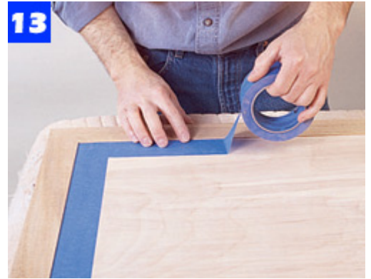
With the edging in place, mask the plywood panel to keep the finish from getting on the surface.
