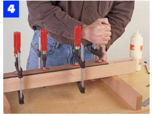
4 Mark the panel positions on each leg, spread glue on the back of a panel, and clamp until the glue sets.
