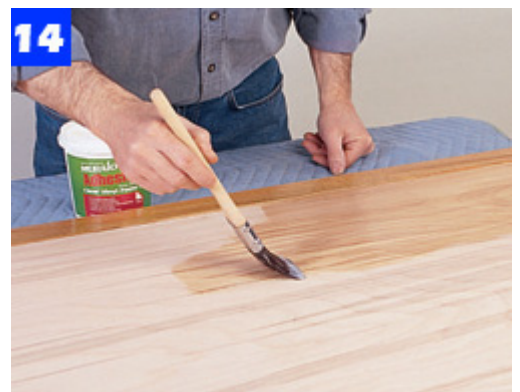
After finishing the edging, spread vinyl wallpaper paste on the panel. Allow it to dry, then apply a second coat.
