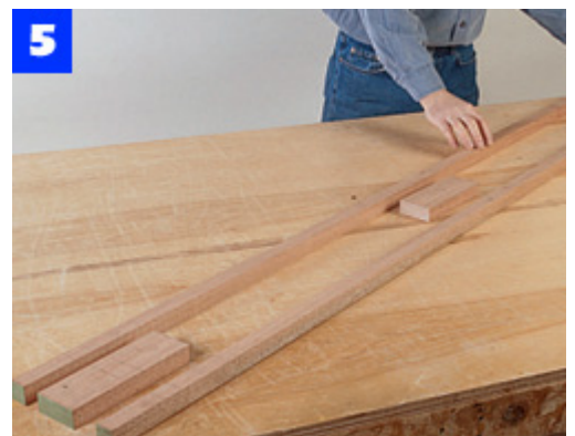
5 Rip three consecutive strips for the drawer apron. Cut the wider middle strip for the center and end sections.
