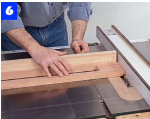
6 Use a dado blade to cut the tenons on the apron ends. The rip fence acts as a stop to ensure uniform tenon length.
