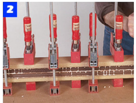
Stack the pieces with paper between each panel and on the top and bottom. Add 3/4-in. cauls and apply clamps.
